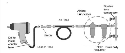
A typical air line layout is shown above. If an automatic in-line filter/regulator is used it will keep the tool in good condition. The lubricator should be adjusted to approx 2 drops per minute and SAE 10 oil should be used.
